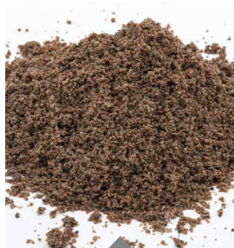
FUGENSPLITT ROT 0 - 3 mm
